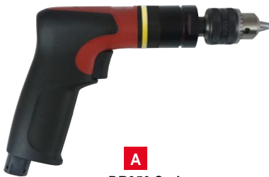
A DR350 Series 350 W (0.5hp) / 550 to 20000 rpm
