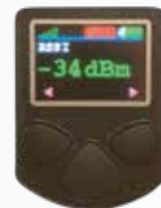
Real-time Wi-Fi signal strength check
