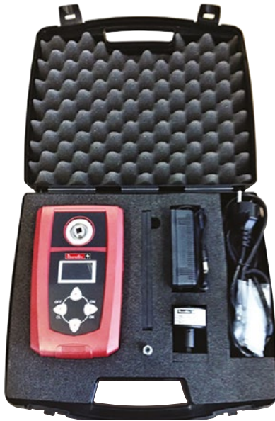
Embedded Transducer & Battery
